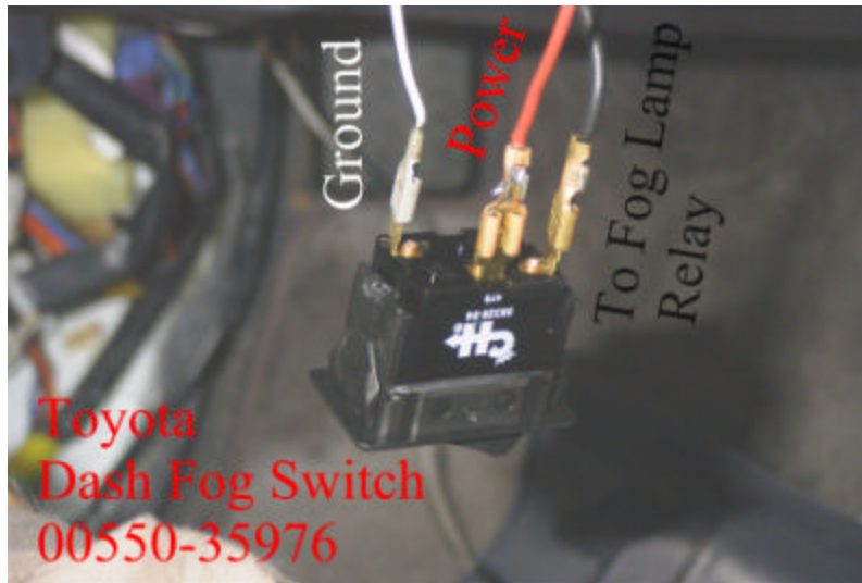
Figure 2 – Fog Switch Detail
